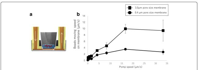
Fig. 3 Analysis of microbead movement on the membrane. a Beads movement tracing experiment. b Bead movement speed alteration depend on pump perfusion volume and membrane pore size
